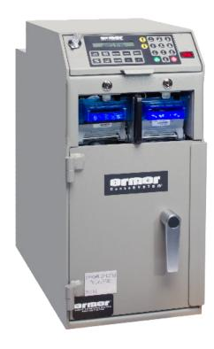
Our CacheSYSTEM® 2400RBH safes feature bill validators that can be removed to clear the occasional bill jam without having to open the safe's main door. While the bill heads are removed, previously deposited notes remain inaccessible as they're securely stored in cassettes inside the safe that can only be retrieved once the safe's main door is open.
